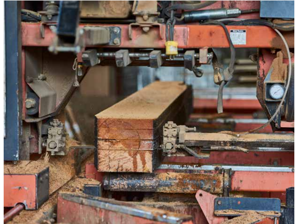
^ > Typical machines at a reclaimed lumber mill: the resaw (above) and industrial planing machine (opposite).
